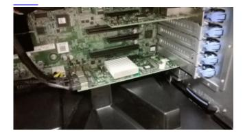
2. Insert new PERC H710 (make sure to plug in the SAS connectors)
